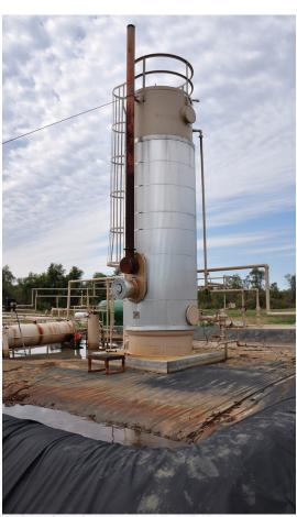
Many industrial and mining processes require chemical basins or lagoons — either for storage, secondary containment or processes such as solvent extraction. Plastatech Oil Resistant (OR) geomembrane is engineered to resist most chemicals — including oils, acid and alkalies as well as a wide range of chlorinated, aromatic and aliphatic hydrocarbons.
